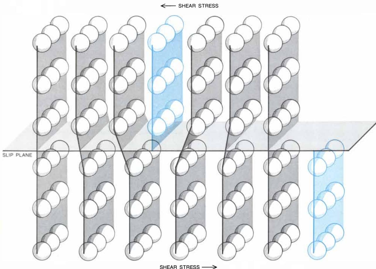
**ROLE OF DISLOCATIONS** in the mechanism of slip is portrayed. The dislocation shown is an extra half plane of atoms (dark color) in the crystal lattice. Deformation occurs by shearing along a slip plane that is perpendicular to the extra half plane of atoms. If shear stress
