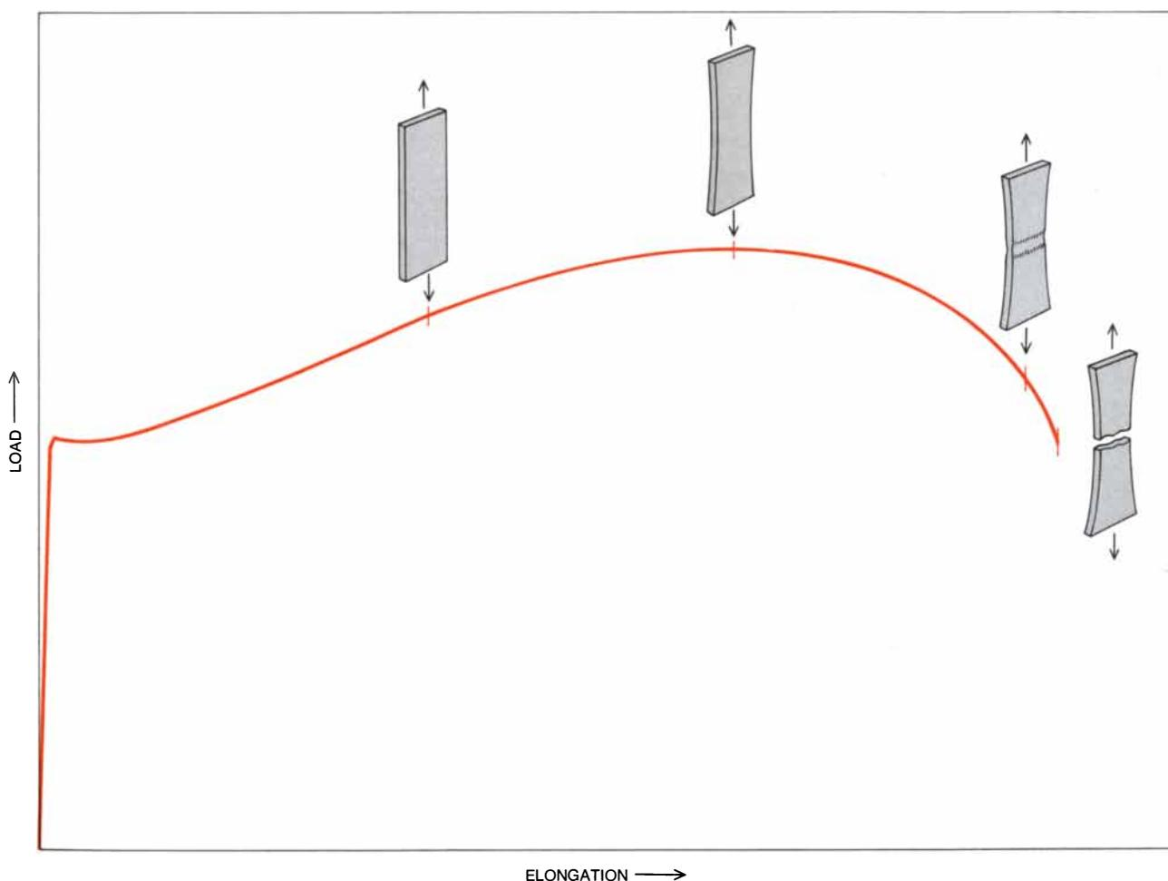
**ELONGATION UNDER LOAD** is tested by pulling a piece of sheet metal to failure in tension. The point where the colored curve turns to the right is the yield point; thereafter the shape of the metal changes permanently. Beyond that point the metal continues to harden as it elongates, so that it is able to carry an increasing load. This intrinsic hardening, termed strain hardening, counteracts the
