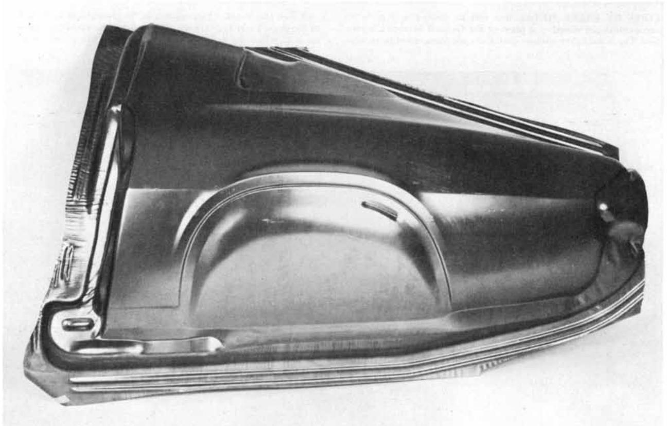
**STAMPED PART** appears as it comes from the stamping press. The part is a "quarter panel" for the left rear side of an automobile; the arched area at the center, which will be over the wheel, will be removed in a trimming operation, as will much of material around the edges and at the right end, where the tail light will be. The material at the edges was for holding the blank in the press as it was stamped.
